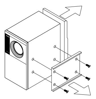
With bass port facing downward, 3 place plenum box over FreeSpace Module being sure to line up access panel in box
