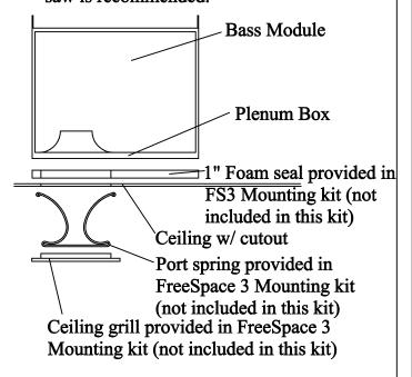
Calculate weight load per local code using a box weight of 30 lbs. Suspend at 4 outside points as well as the center safety point.
