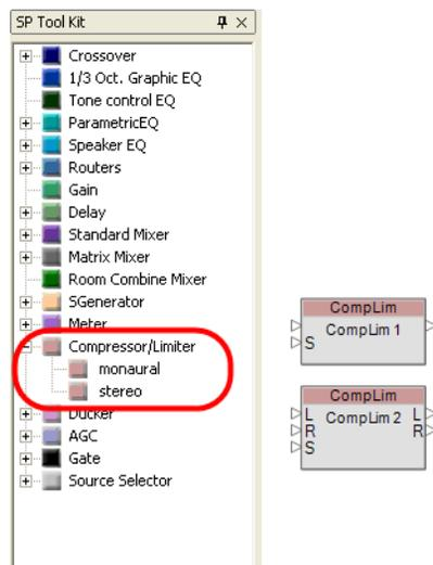
Figure 7.51 - Compressor/Limiter
