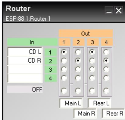
Figure 7.27 - A stereo input routed to four different outputs
