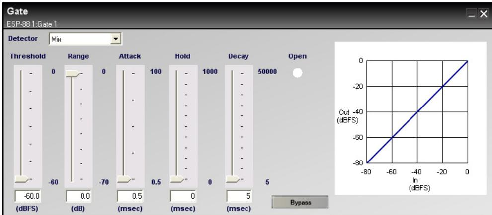
Figure 7.58 - Gate control panel
