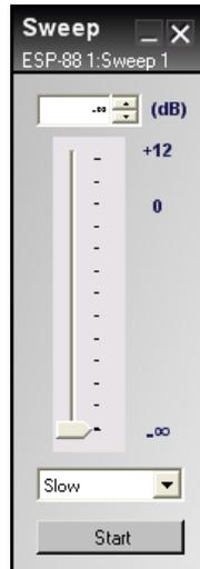
Figure 7.48 - Sweep generator control panel
