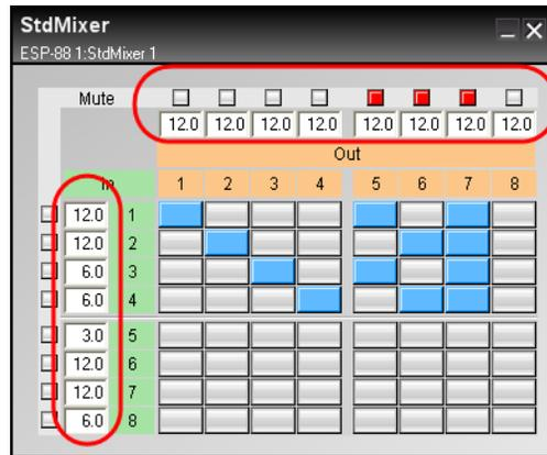
Figure 7.35 - Adjust input and output levels
