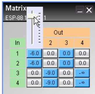
Figure 7.38 - Right click on an assign button to adjust gain
