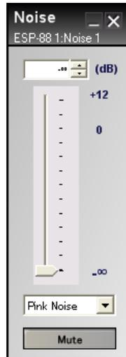
Figure 7.47 - Noise generator control panel
