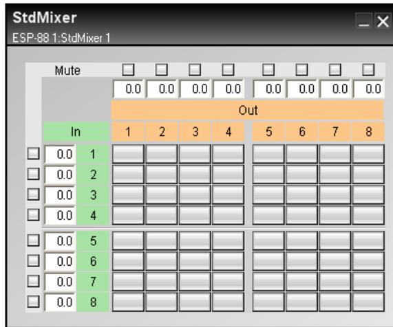
Figure 7.33 - 8X8 standard mixer control panel
