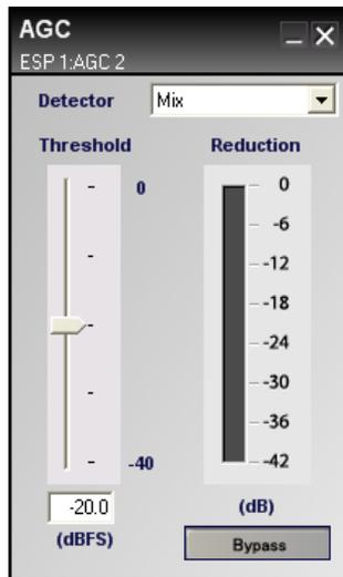
Figure 7.56 - Stereo AGC control panel
