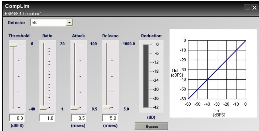
Figure 7.52 - Stereo Compressor/Limiter control panel
