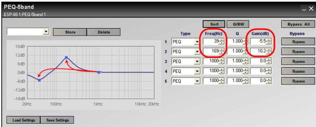
Figure 7.14 - Drag the blue boxes to set frequency and gain
