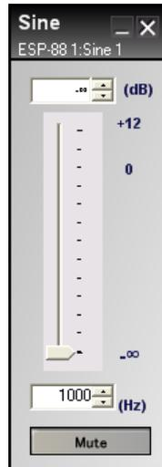
Figure 7.46 - Sine wave generator control panel
