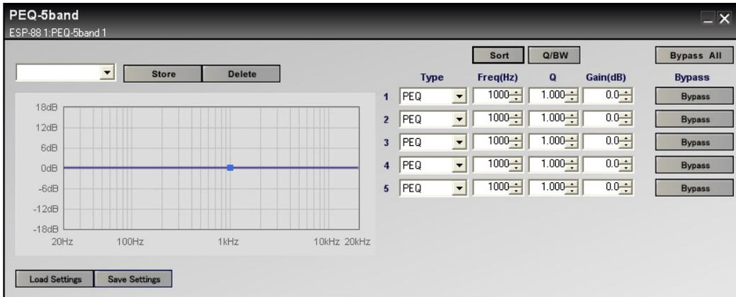
Figure 7.13 - 5 band Parametric EQ control panel
