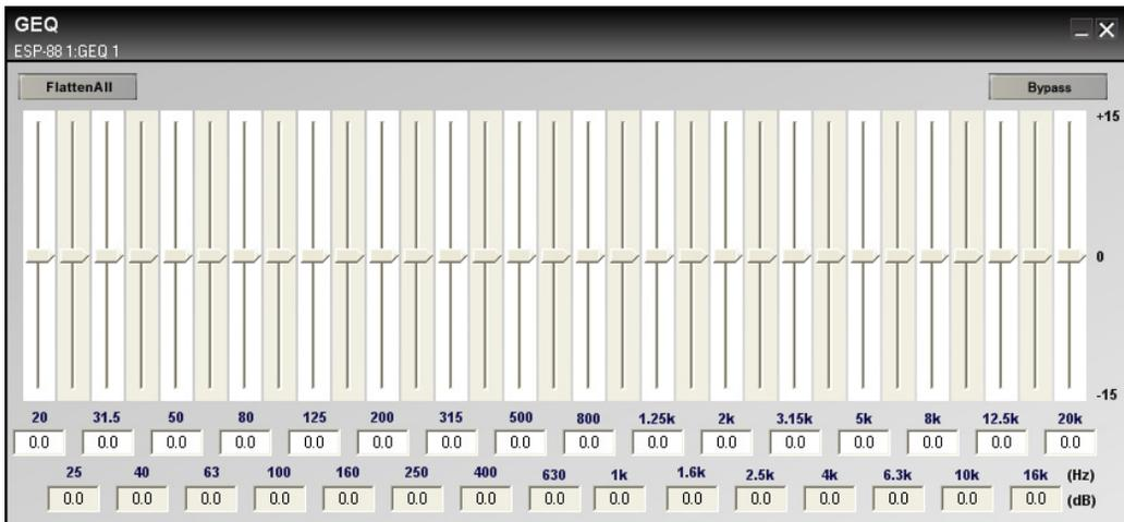
Figure 7.9 - 1/3 Oct Graphic EQ control panel
