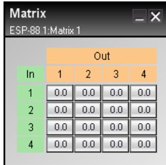
Figure 7.37 - 4X4 matrix mixer control panel
