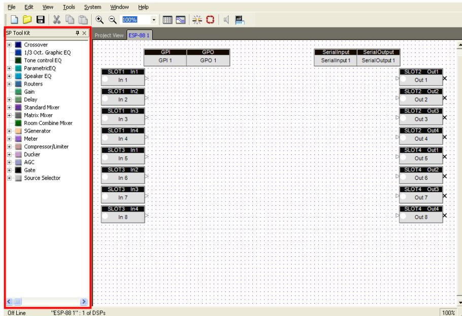
Figure 7.1 - ESP-88 window with SP Tool Kit to the left
