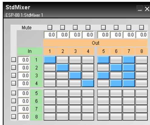
Figure 7.34 - Press the assign buttons to route inputs to outputs
